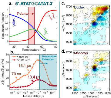
Fig 1. (a) Population profile demonstrating multistate dissociation (b) t-HDVE time traces showing initial fraying of the AT ends of the duplex. 2D IR spectra of DNA (c) duplex and (d) monomer.
